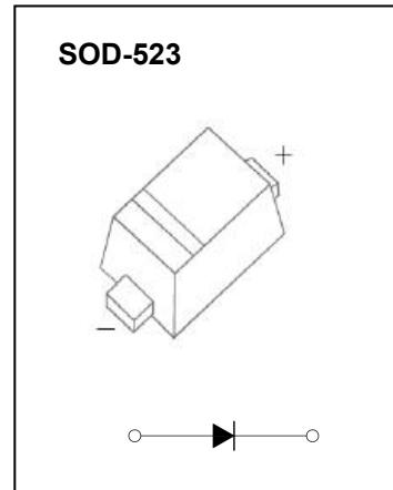
**Maximum Ratings and Electrical Characteristics, Single Diode @Ta=25°C**
