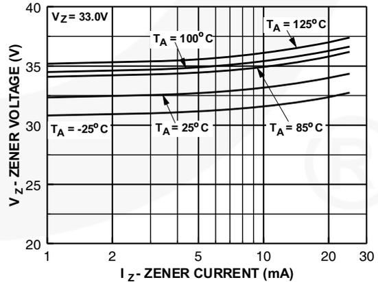
Figure 6. 33 Zener Voltage vs. Zener Temperature
