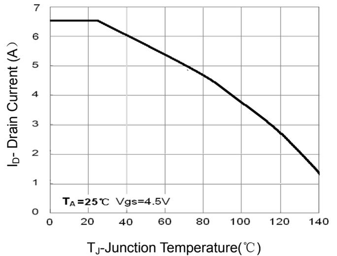
Figure 4 Drain Current
