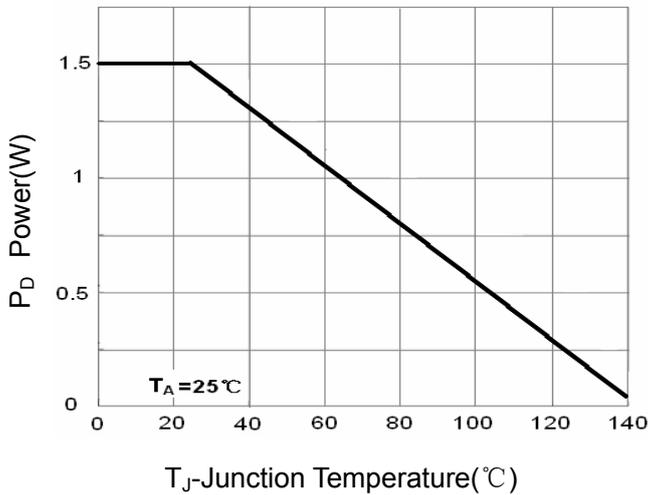
Figure 3 Power Dissipation
