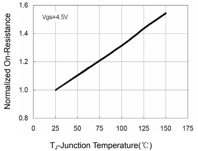
Figure 8 Drain-Source On-Resistance
