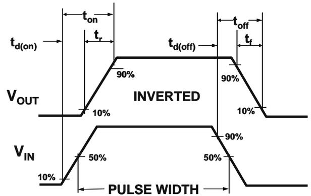
Figure 2: Switching Waveforms
