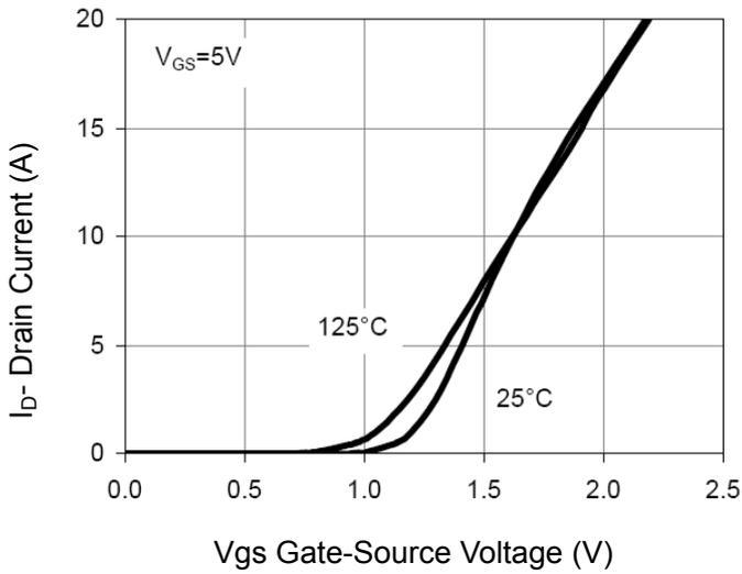
Figure 7 Transfer Characteristics
