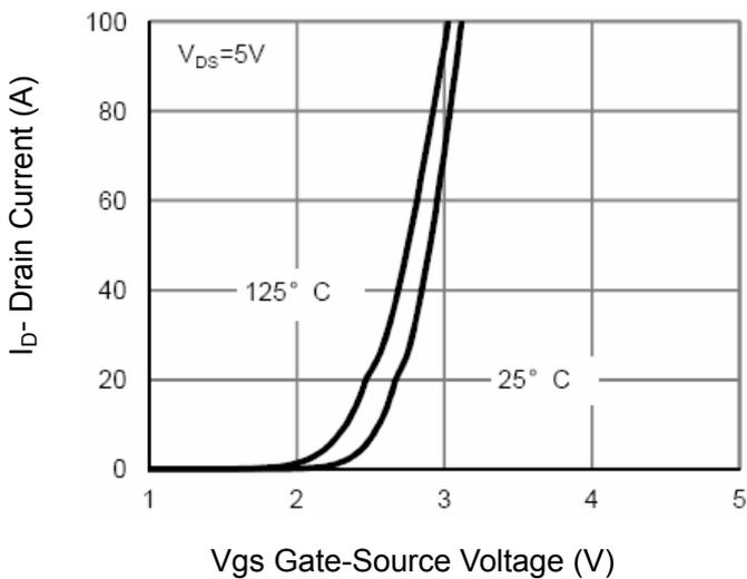
**Figure 2 Transfer Characteristics**
