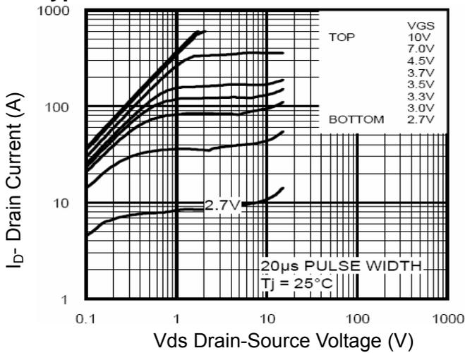
Figure 1 Output Characteristics
