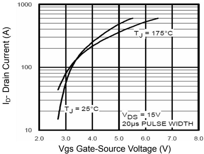
Figure 2 Transfer Characteristics
