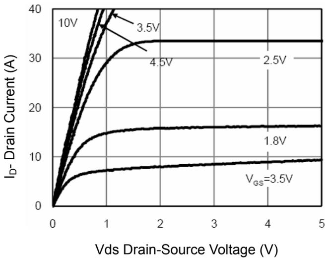
Figure 3 Output Characteristics
