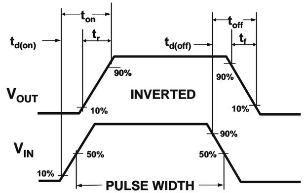
Figure 2: Switching Waveforms
