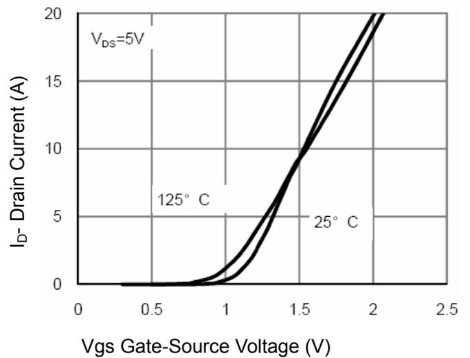
Figure 4 Transfer Characteristics
