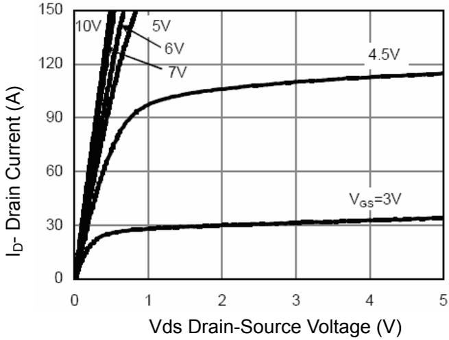
Figure 1 Output Characteristics
