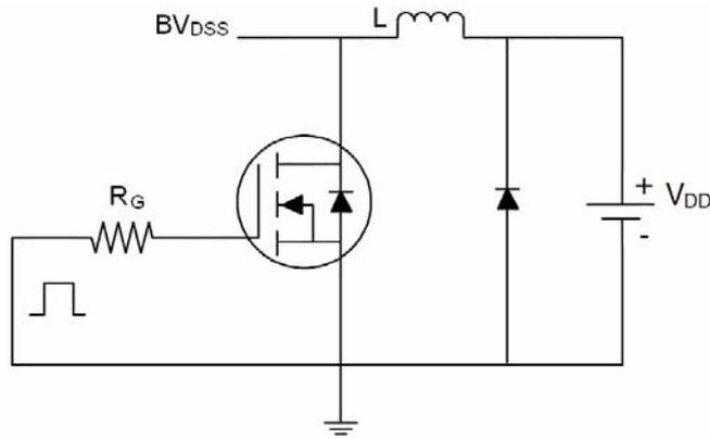
2) Gate Charge Test Circuit
