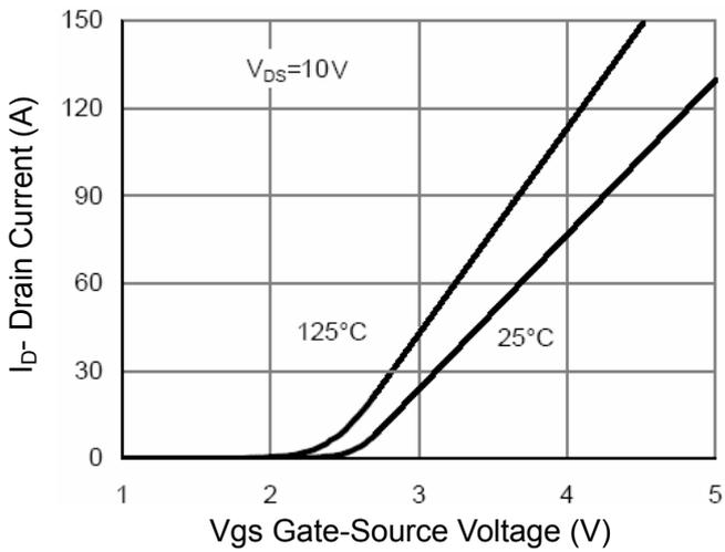
Figure 2 Transfer Characteristics
