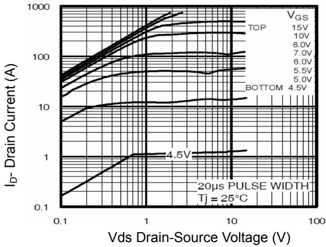
Figure 1 Output Characteristics
