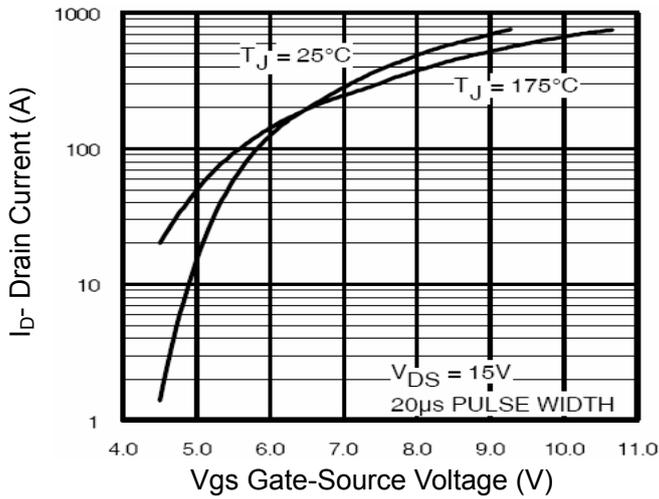
Figure 2 Transfer Characteristics
