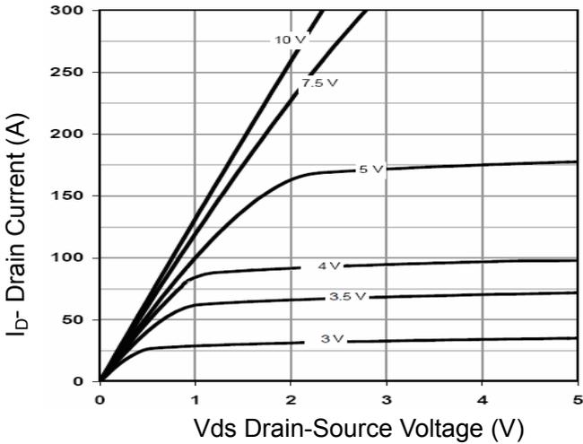
Figure 1 Output Characteristics
