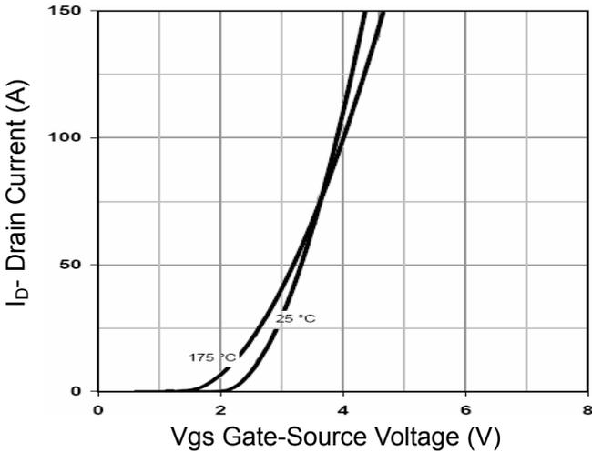
Figure 2 Transfer Characteristics
