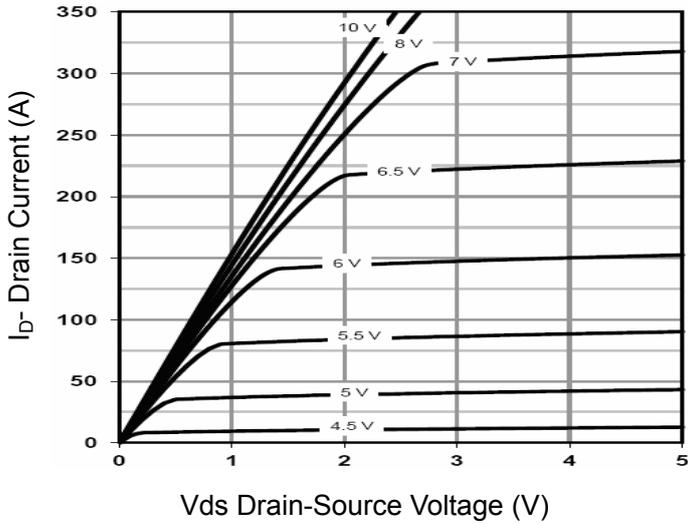
Figure 1 Output Characteristics
