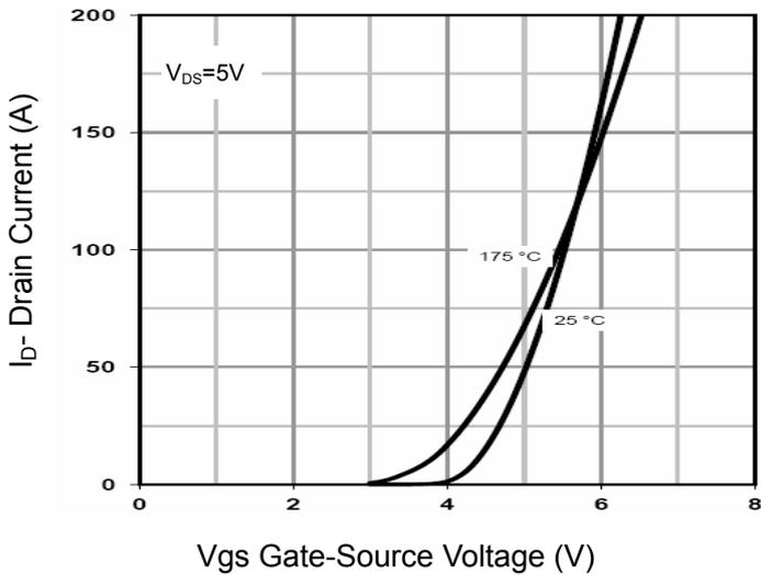
Figure 2 Transfer Characteristics
